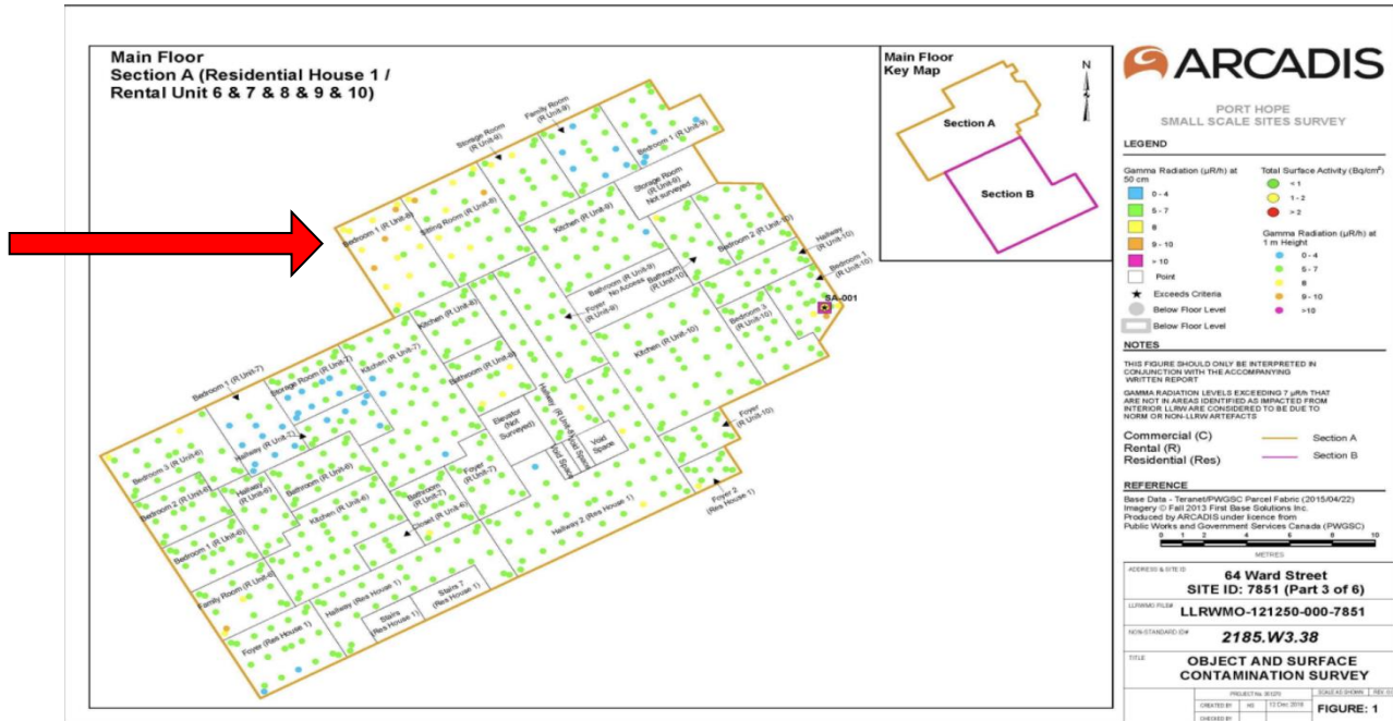
Figure 3: ARCADIS Design and Consultancy Survey of Radioactive Contamination on the North Side of 64 Ward Street. 27
