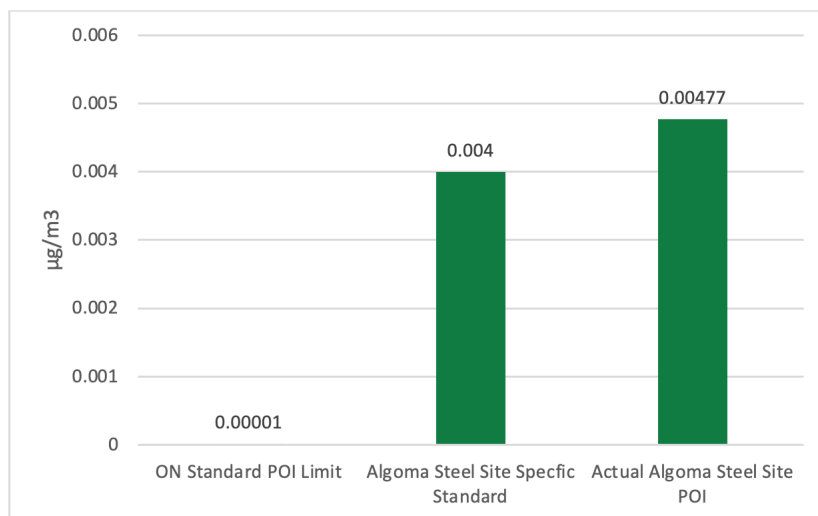
Figure 2: A comparison of the Ontario and Algoma Steel site-specific standard for benzo(a)pyrene, and the actual benzo(a)pyrene emissions in 2020.
