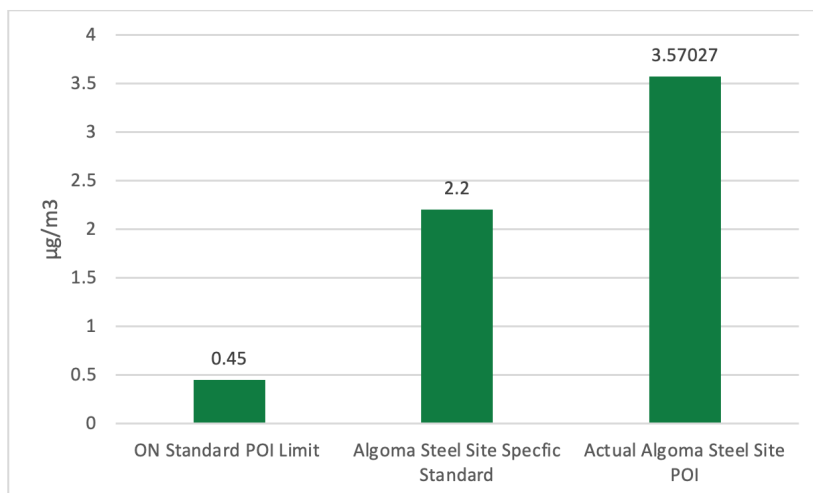
Figure 1: A comparison of the Ontario and Algoma Steel site-specific standard for benzene, and the actual benzene emissions in 2020.
