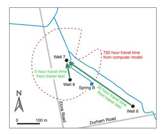
Figure 3 Trajectories and travel times for the tracer tests started on October 29th 2001, showing velocities >300 m/day, compared to a 30 day capture zone predicted using MODFLOW (Worthington et al., 2001b).
