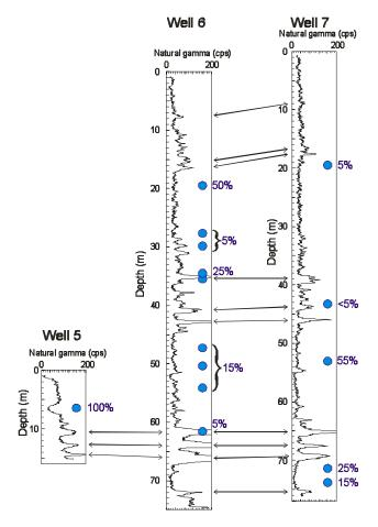
Figure 2 Stratigraphic correlation of Wells 5, 6, and 7 using gamma logs, showing the major locations of inflow to the wells (after Worthington et al., 2000a)
