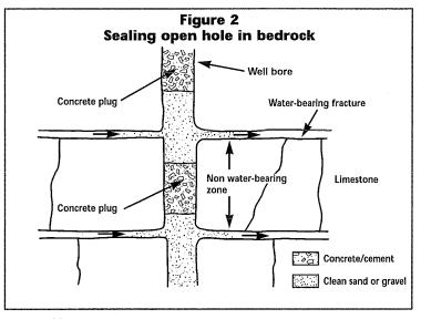
the wall of the borehole, and provide the most effective seal against moving water. If alternating cement or concrete plugs and sand and gravel are needed to control the groundwater movement, the concrete plugs must be placed in known non-producing, competent horizons. If the location of the non-producing horizons is not known, place plugs at sufficiently frequent intervals to ensure an effective seal.
